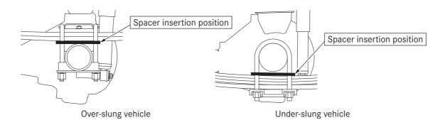
Remove the center bolt of the spring, then while referring to the table below select a suitable number of spacers, insert them, and retighten the center bolt to the specified torque.
