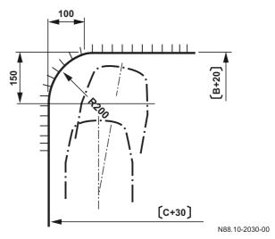
Note: The fender must not be inside the shaded area.
