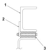
Installation of out-of-position preventive retainer
