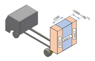
\*2) Distance from the rear end of the vehicle, including the body, to the tip of the camera lens
