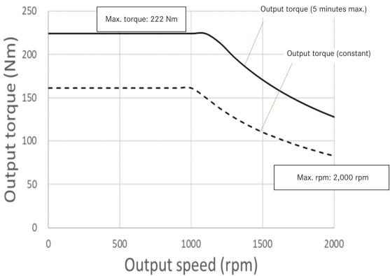
· Performance curve diagram of ePTO with pulley
