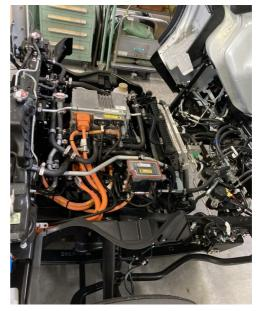
Space where HV components are located (under cabin)
