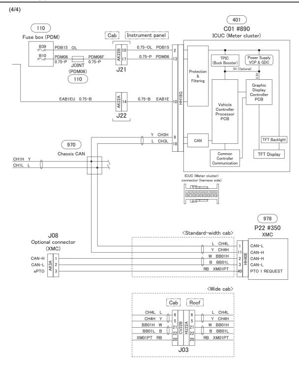
CAN : Controller area network ePTO : Electric power take off XMC : Expansion module cabin
