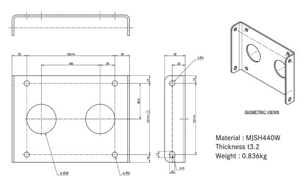
3. ALL PARTS MUST BE FREE FROM CRACK AND BURRS.2. CORNER RADIUS MUST BE R10 UNLESS OTHERWISE SPECIFIED.NOTE 1. INSIDE BEND RADIUS MUST BE R5, UNLESS OTHERWISE SPECIFIED.
