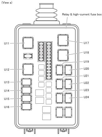
U11 Vacuum pump relay 2 U12 VCU main relay A/C S/OFF valve relay U13 U14 Condenser fan relay 2 U15 3/2-WAY valve relay (HVB) U16 Condenser fan relay 1 U17 Electric parking lock (EPL) relay Vacuum pump relay 1 U18 U19 KL15 VTL relay U20 Water pump relay (HVAC) U21 Water pump relay (Motor) U22 Chiller S/OFF valve relay U23 Air-conditioner clutch relay U24 Water pump relay (HVB)
