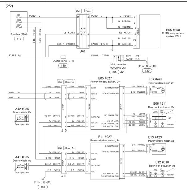
As: Assistant driver's seat side CAN: Controller area network Dr: Driver's seat side ECU: Electronic control unit LIN: Local interconnect network
