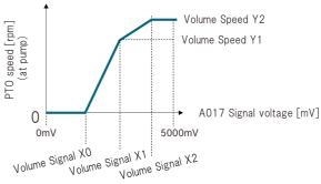
If Target Speed XXXX[rpm] is not "0", volume speed control will be changed as shown in figure.
