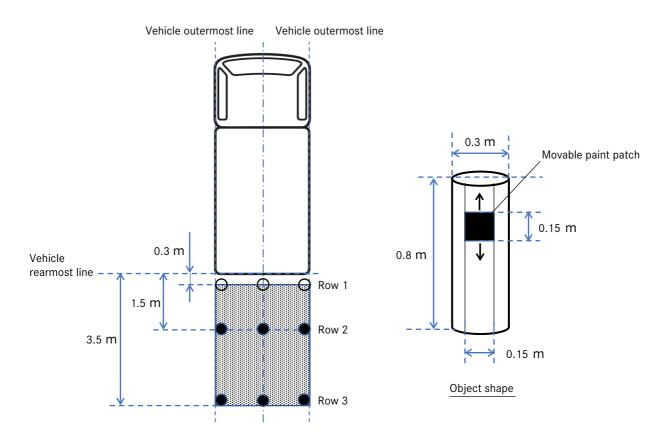
Row 1: The paint patch (area of 0.15 m  $\times$  0.15 m) or the top surface of each object must be visible.
