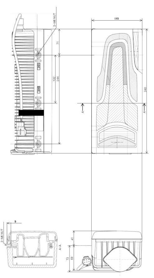
• Installing the rear combination lamp, attach it to the combination lamp mounting hole. Keep the bolt fitting part 9 mm or less.
