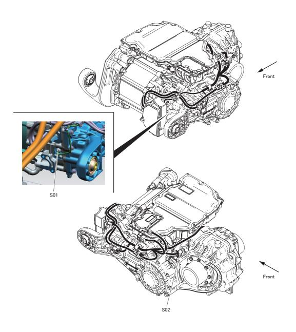
S01 Parking gear switchS02 Vehicle speed sensor
