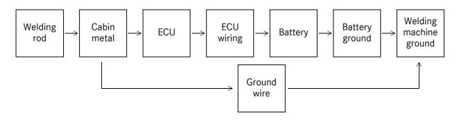
As a result, other wiring including the ECU and the ground wire will be damaged.
