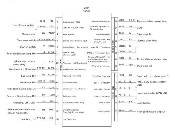
ASAM: Advanced signal detect and actuation module
