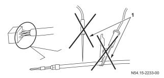
1 Sticking of test bar or electric circuit check lamp needle into cable insulation is prohibitive.
