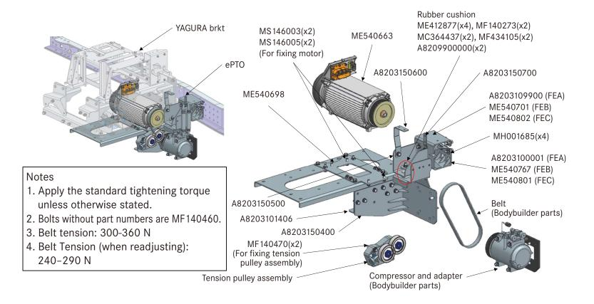
Tension pulley assembly
