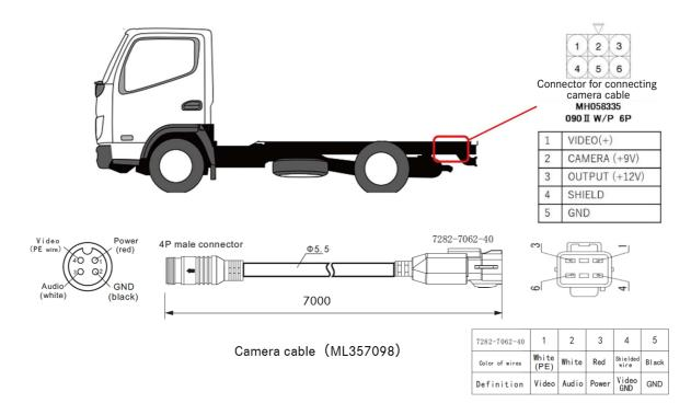
(c) Arrange for an extension cable if the length is insufficient.
