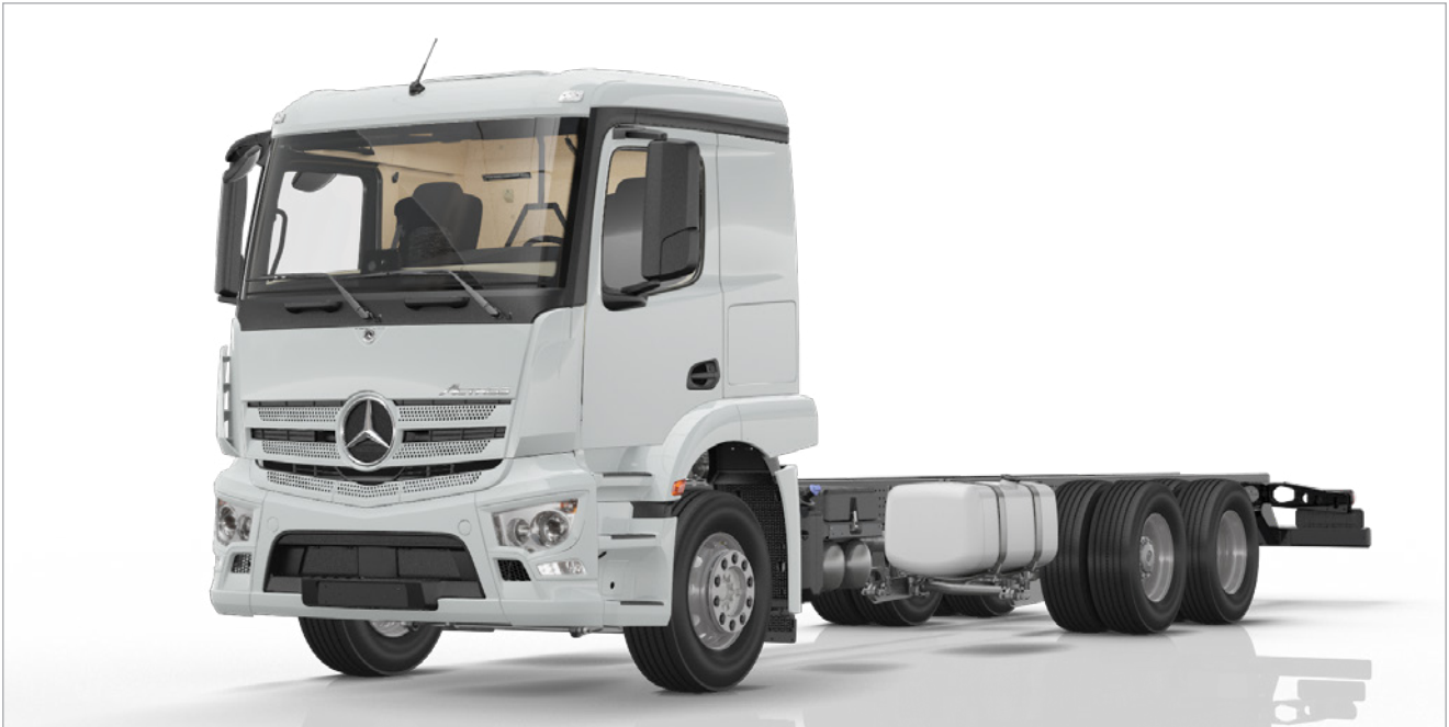
L-Cab ClassicSpace 2.30m, tunnel 320mm
